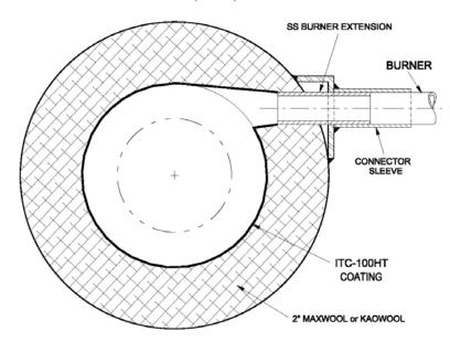
VERTICAL CYLINDER FORGE OR CRUCIBLE FURNACE
