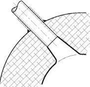
The end of the burner tube should be no closer to the inside of the forge than 1" (25mm) or excessive burning of the of the tube will result.
